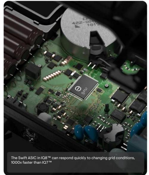
The Swift ASIC in IQ8™ can respond quickly to changing grid conditions, 1000x faster than IQ7™
